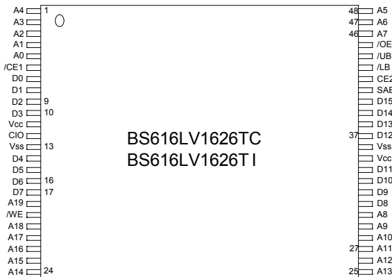
48-pin 12mmx20mm TSOP1 top view
