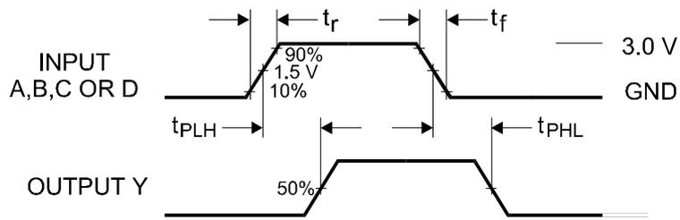
**Figure 1. Switching Waveforms**
