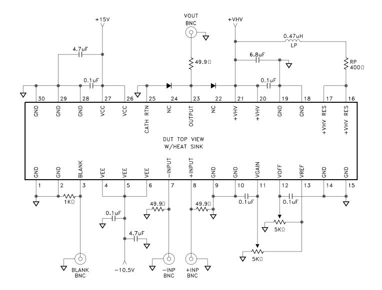
The connection circuit shown above is for the MSK 1902-0 evaluation board. The Rp and Lp are external components and must not be located near ground planes if possible. A high quality resistor such as Bradford Electronics P/N FP10-400 is required for optimum response times. Use an inductor with a high self-resonant frequency that can withstand the currents required for the application.
